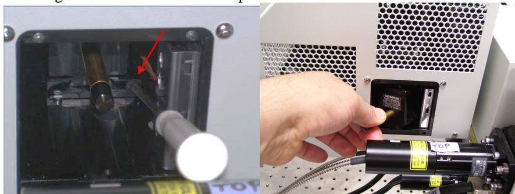
4) Carefully put the cube in a plastic bag and in the appropriate box. Do not touch the filters!
