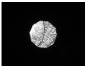
D: Field Diaphragm focused and centered
