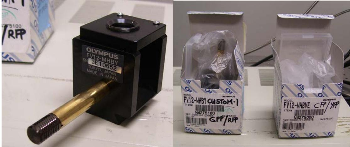
5) Put a new filter cube in place. The dovetail on the bottom of the cube has to slide into the matching track in the housing. Gently push the cube all the way in until you hit the end wall (be careful, no slamming).
