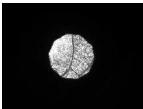
D: Field Diaphragm focused and centered
