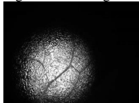
B: Field Diaphragm closed down, not focused, not centered
