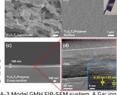
focused ion beam (FIB) milling with a Tescan FERA-3 Model GMH FIB-SEM system. A Ga+ ion beam was used to mill the samples after depositing protective Pt layer over the region of interest. Find more information about sample prep on the MIC website. The samples and images were submitted by Yang Hyun Auh from Dr. Jodie L. Lutkenhaus's Lab in Chemical Engineering and are courtesy of Dr. Kailash Arole, Dr. Yordanos Bisrat and Dr. Sisi Xiang.
